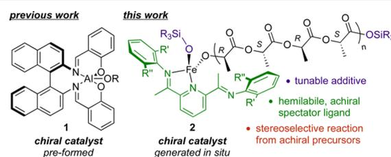
**Figure 1.** Strategies for catalysts designed to synthesize stereoregular PLA.
