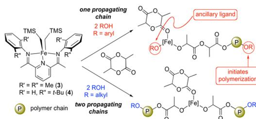
dimethylphenyl bis(imino)pyridine iron precursor **3** as originally reported,<sup>11</sup> the level of stereoselectivity in lactide polymerization was improved when silanols were used as additives, albeit with less control over polymer molecular weight. Compared to atactic polymer produced from reactions initiated with *p*-methoxyphenol (Table 1, entry 1), polymerization of (*rac*)-lactide initiated by a mixture of **3** and Ph<sub>3</sub>SiOH led to slightly heterotactic PLA (entry 2).
