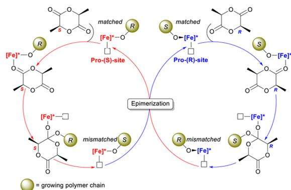
**Figure 5.** Mechanism for heterotactic polymerization of (*rac*)-lactide. The Cahn–Ingold–Prelog designation in the polymer chain represents the stereocenter proximal to metal.
