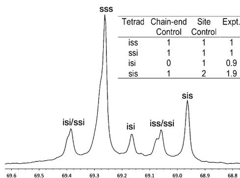
**Figure 2.** <sup>13</sup>C{<sup>1</sup>H} NMR spectrum of PLA obtained from Table 1, entry 9. The table contains experimental and predicted distribution of stereoerrors from chain end and enantiomorphic site control mechanisms (*s* = syndiotactic, *i* = isotactic).
